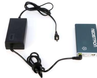
Plug the power connector from the Apex ICH / Resvent iBreeze AC adapter into the Charge Port of the Pilot-24 Lite and plug the other end into the power outlet.
